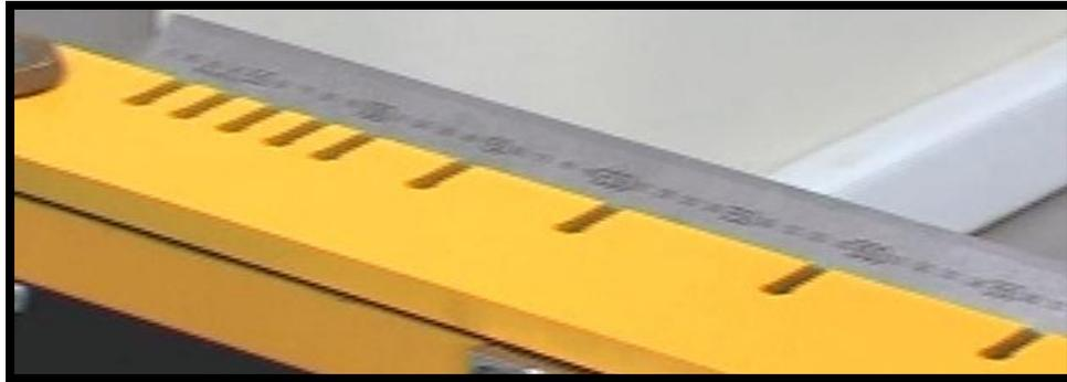
Measuring the slotted clamp bar
