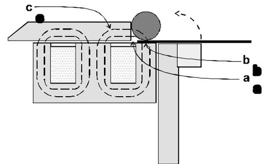
2. Wrap the sheet metal around the rolling bar as far as possible –
