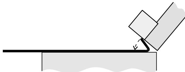
3. Further flattening can be accomplished when using thin lightweight material by following up with magnetic clamping
