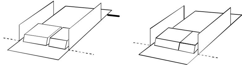
Select the largest clamp piece for bends up to 70mm and for longer lengths use several clamp pieces to fit the required length.
